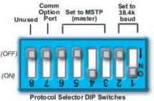
Fig. 67 - RTU-MP SW3 Dip Switch Settings
